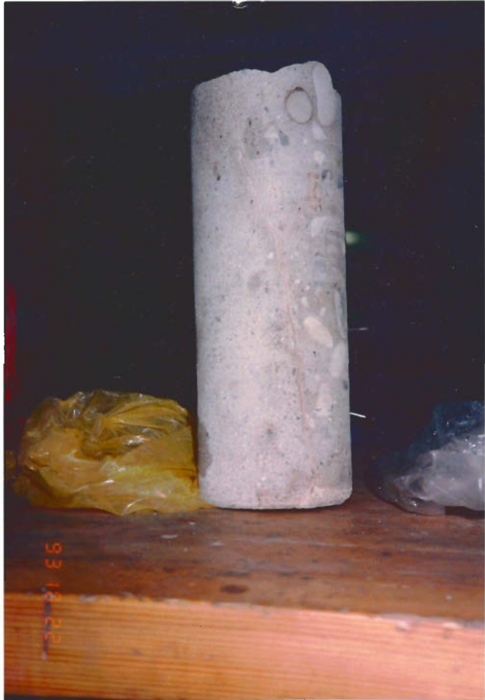
Figure 3.13 Core from injected crack. The crack was injected with polyurethane.
