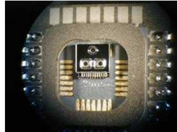
Sensor chip area: 3 x 3 mm. Packaged in a standard ceramic package
