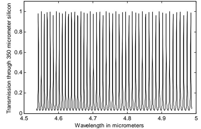
Absorption pattern synthesized by multi-line filter
