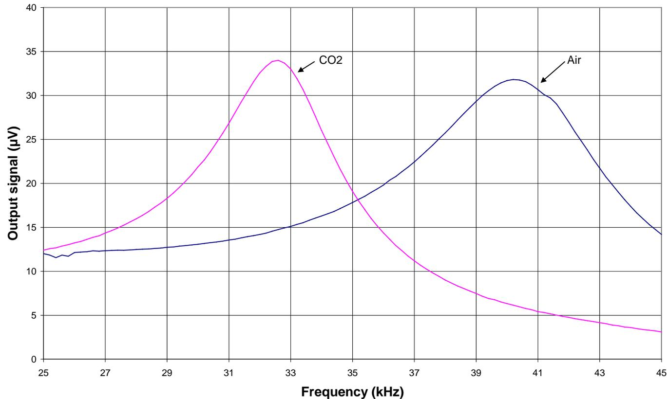
The resonance frequency shifts from 40 to 32 kHz and the Q factor increases from 6.5 to 8.1
