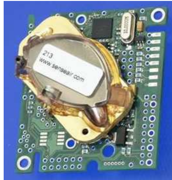
SenseAir infrared CO 2 sensor for embedded solutions
