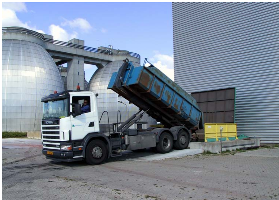
Figure 2. Transfer of sludge cake from Damhusåen WWTP to the incineration plant at Avedøre WWTP. 2006-08-10.
