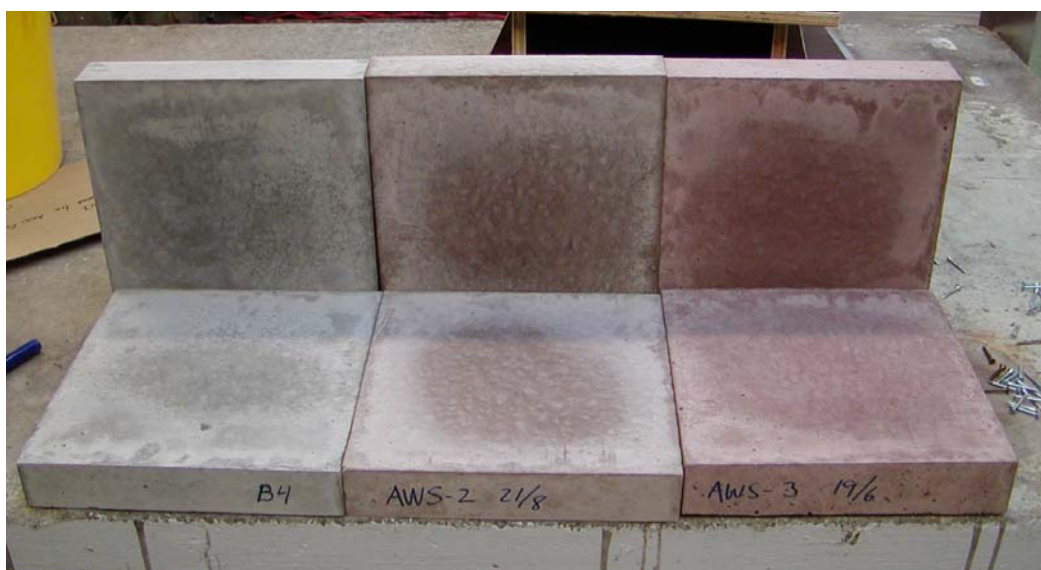
Concrete slabs with 1) no bio ash, 2) light bio ash and 3) red bio ash
