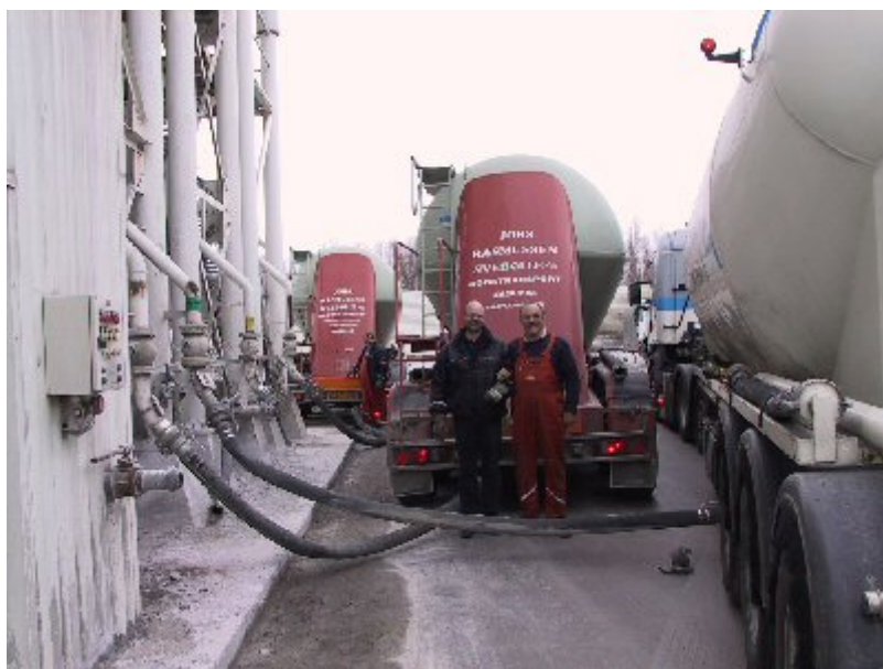
Unloading bio ash at Unicon's plant in Avedøre.
