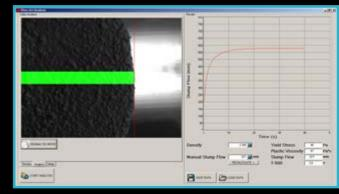
The system is a PC automated slump flow test where the flow curve (spread vs. time) is determined using digital image analysis. The flow curve is used to determine yield stress and plastic viscosity.
