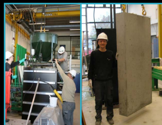
Left: Casting of large concrete block at the DTI laboratory.
