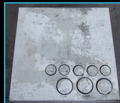
Cores ( \varnothing 100 and \varnothing 150 mm) are drilled from concrete blocks at 28 days of maturity.
