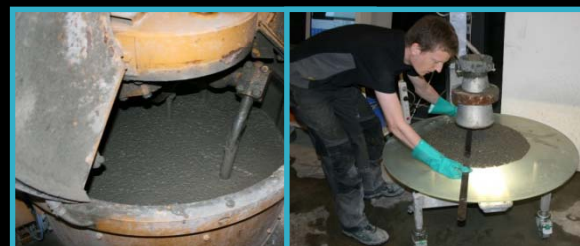
Left: Self-compacting concrete in the mixer.
