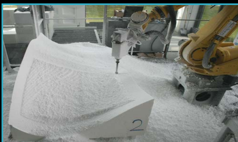
Industrial robot cell at the Concrete Centre, milling out a double curved formwork shell guided by CAM software.
