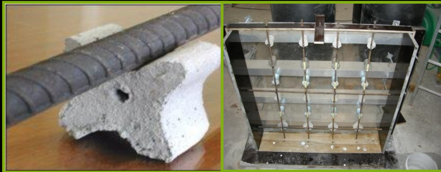
Bone shaped concrete spacer tested by DTI
