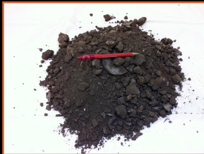
Sample of bottom ash from incinerated municipal waste.
