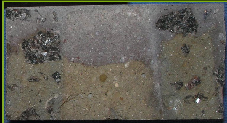
Chloride migration tests was performed on the spacers. The silver nitrate used for the test has penetrated much farther into the spacer than anticipated indicating a very porous structure.
