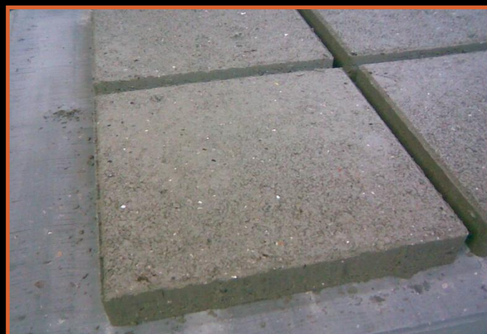
Pavers produced with zero slump concrete containing bottom ash.
