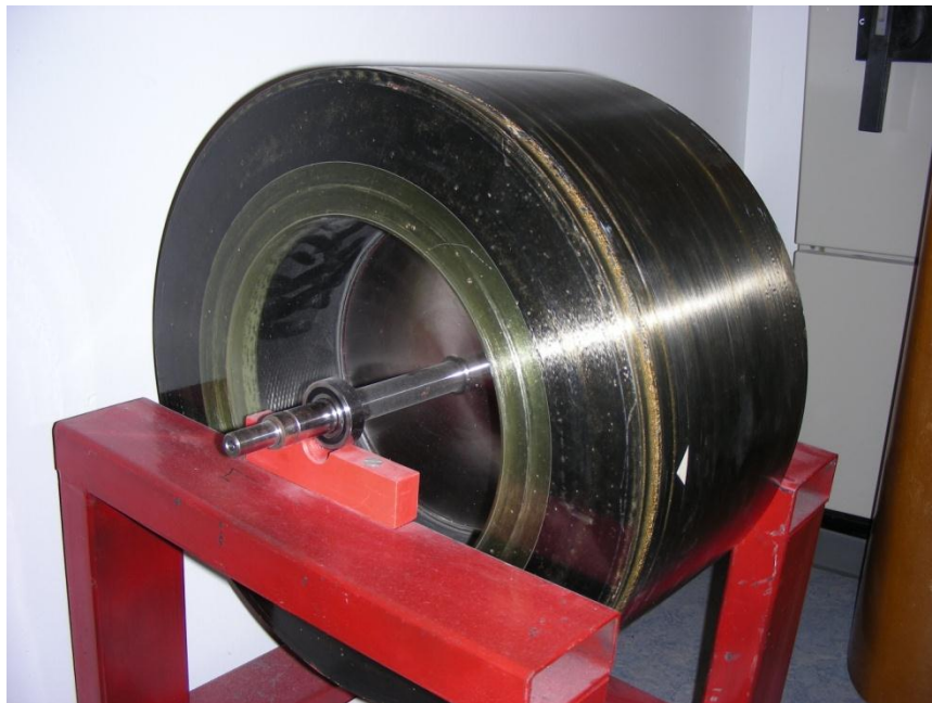
Figure 3.3.1. Small laboratory flywheel developed in the early nineties at Risoe and intended for mobile use in vehicles. The weight is 22 kg and the storage capacity at 36000 rpm is 4.6 MJ or 1.3 kWh. The power is in the range of 500 kW.
