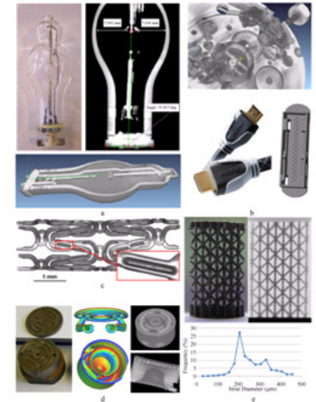
Figure 2. Typical part calling for CT metrology: a) Measuring equidistance and electrode distance in multi-material lamp bulb; b) Multi-material assembly/inclusion (with lead connector); c) Measuring drug eluting cavity in stent; d) Layered manufactured mesh with complex internal channel; e) Measuring beam thickness in medical bone scaffold.
