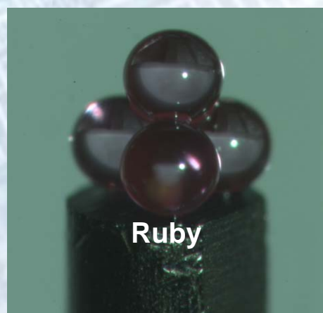
Microtetrahedrons with 3 ruby spheres and one sphere of different material (all Ø 0.5 mm)
