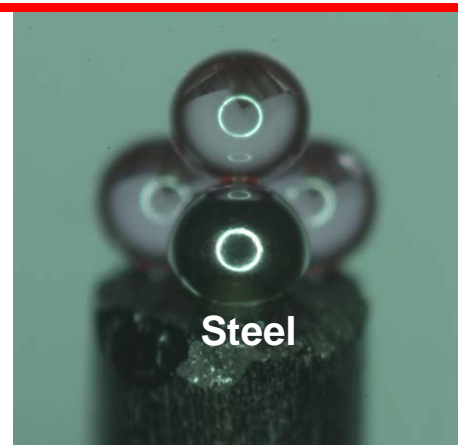
Microtetrahedrons with 3 ruby spheres and one sphere of different material (all Ø 0.5 mm)
