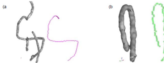
3D visualization of two single fibres showing the gray value data on the left and the extracted medial axis in colour on the right
