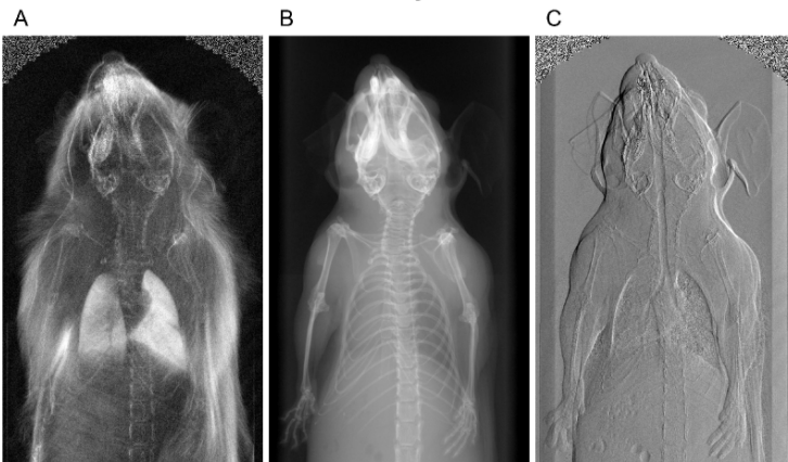
Fig 5: In Vivo X-Ray Dark Field, Absorption and Phase Contrast Projection of a Mouse
