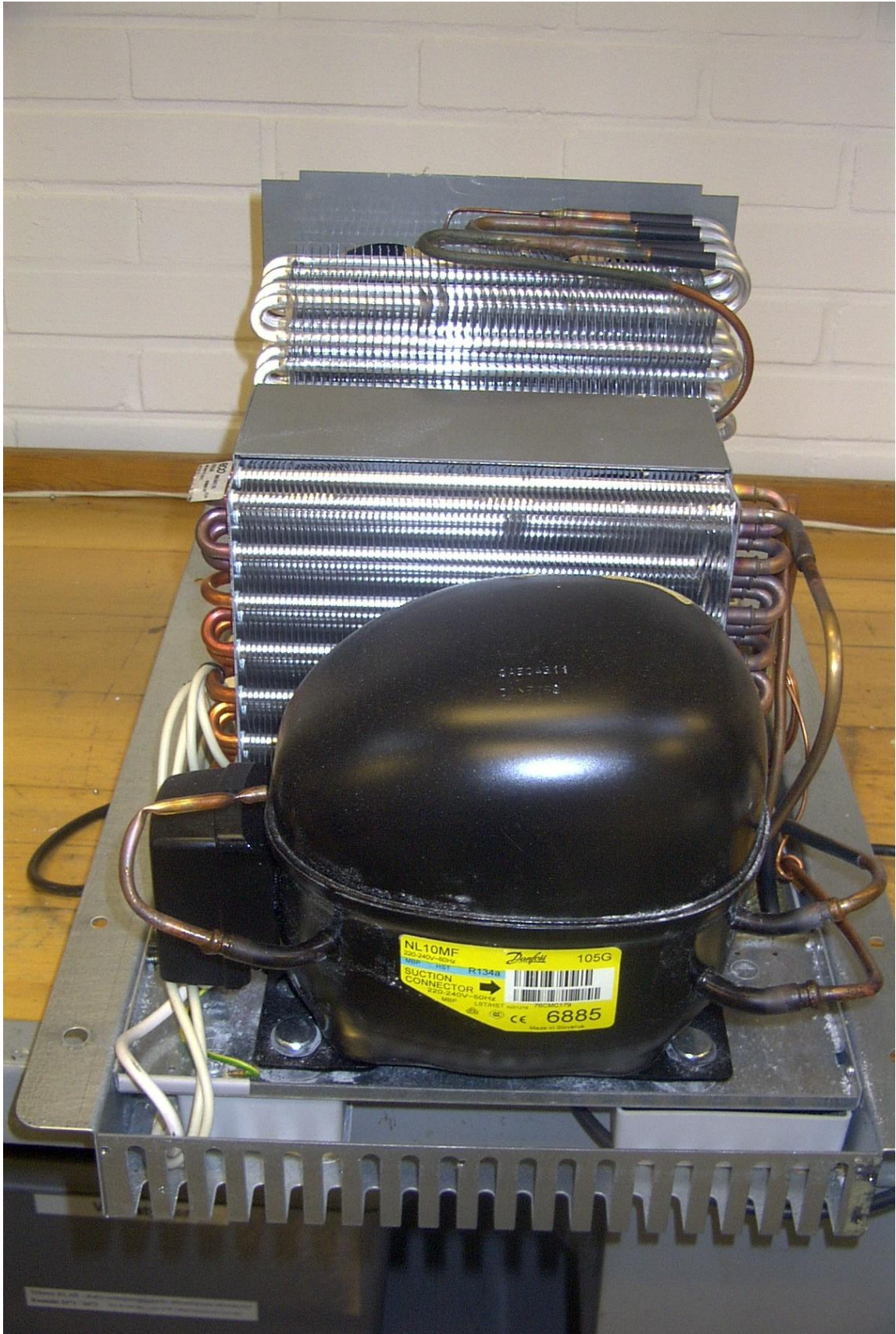
Figure 9: The refrigeration system after dismantling of insulation and steel enclosure.
