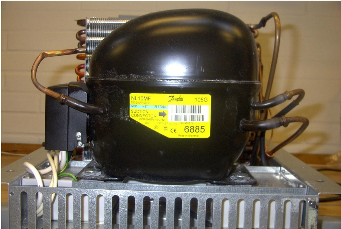
Figure 10: The compressor: NL10MF from Danfoss. R134a.
