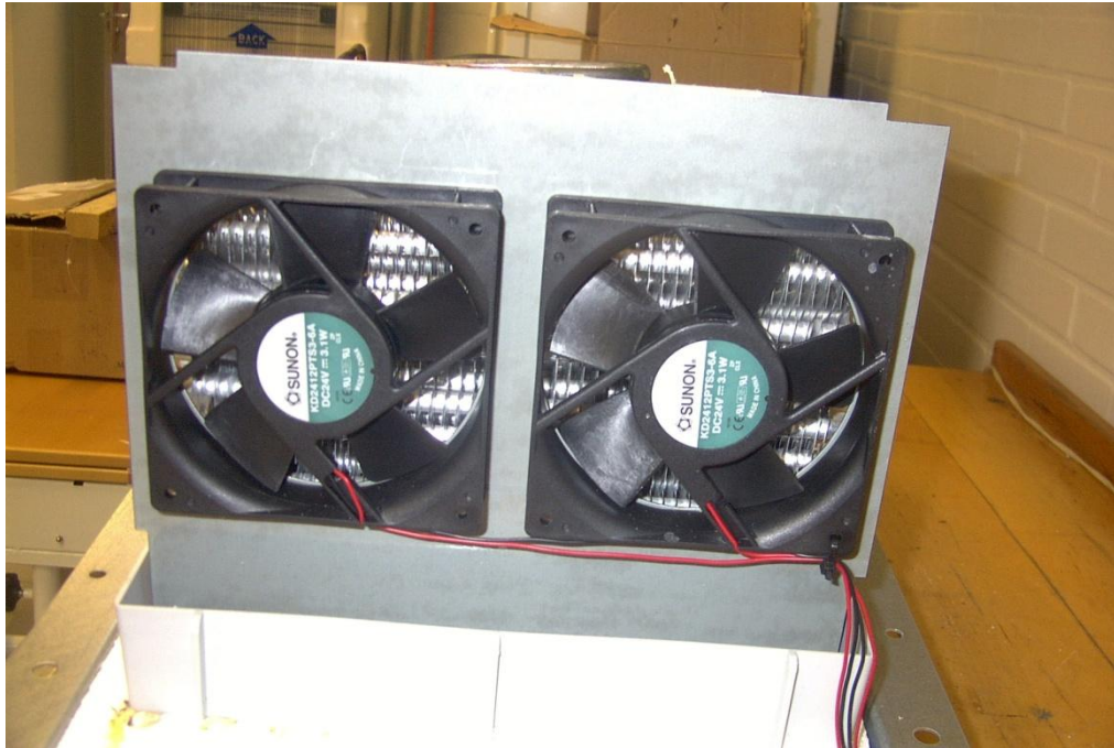
Figure 12: The two DC fans on the evaporator.
