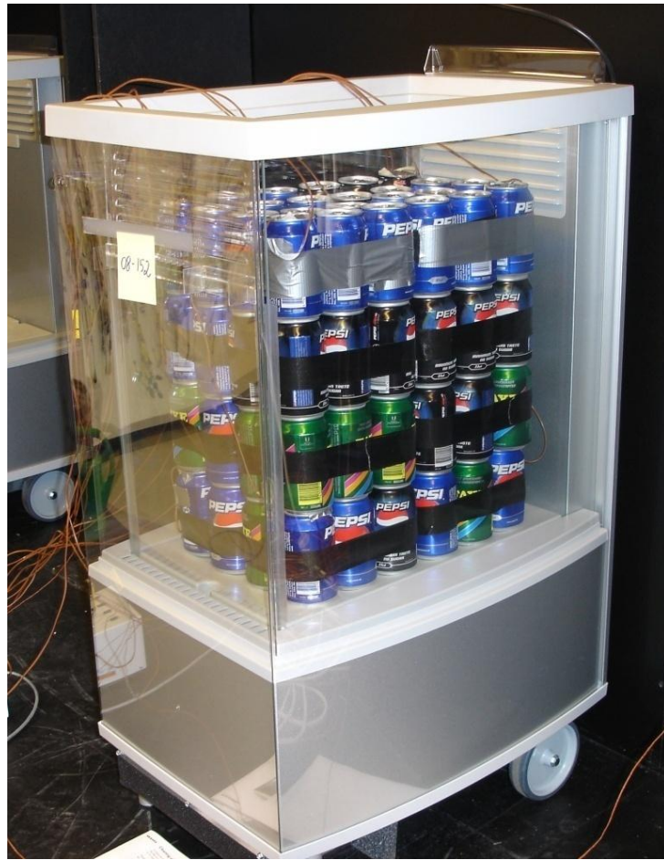
Figure 15: In test 2 and 3 the baseline coolers were tested with cans taped in “six packs” to prevent disorder of the cooling load.
