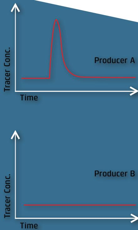
Figur 1. Tracer responses in the two monitored producers. Only Producer A is connected to the injector via a fracture. There are no secondary fractures as only one signal is observed.
