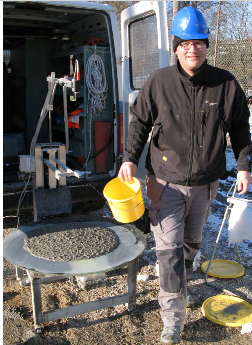
Figure 3.3. Automated slump flow measurement applied during job site quality control. To determine the slump flow and viscosity class (4C-Rheometer).
