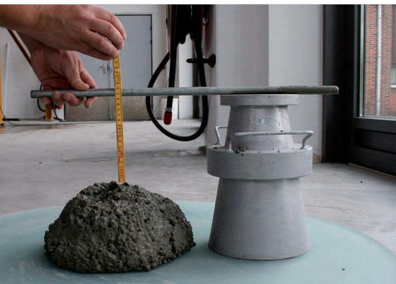
Figure 1.1. The slump value of traditional concrete (left) measured as the setting of a 300 mm high concrete cone. The slump flow measurement of a similar SCC test object is shown on the right. The slump value for traditional concrete is typically in the range of 100-200 mm, while the slump flow for SCC is typically 500-700 mm.
