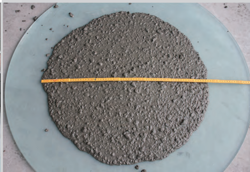
Figure 1.1. The slump value of traditional concrete (left) measured as the setting of a 300 mm high concrete cone. The slump flow measurement of a similar SCC test object is shown on the right. The slump value for traditional concrete is typically in the range of 100-200 mm, while the slump flow for SCC is typically 500-700 mm.
