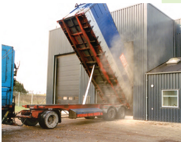
Figure 6. Wood chips unloaded at a Danish district heating plant. Very high concentrations of mould spores
