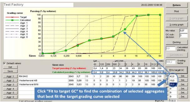
Figure 9. The best fit to the selected target grading curve is the 42:19:39 % by volume combination of RN 0/4 E, Vesterhavsral 4/8 and Vesterhavsral 8/16. The corresponding grading curve is shown as the "Calculated passing (% by volume)" and as the green line on the graph.
