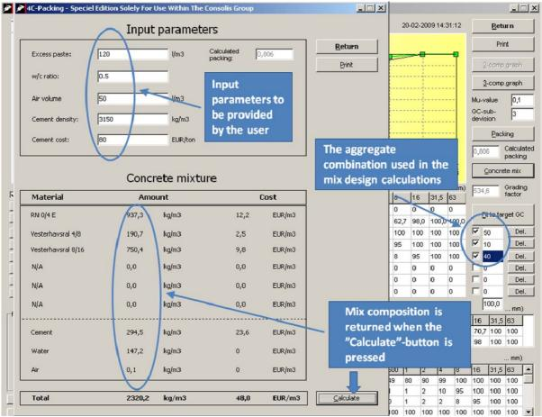
Figure 17. Calculation of concrete mix design based on a 50:10:40 % by volume combination of RN 0/4 E, Vesterhavsral 4/8 and Vesterhavsral 8/16. Add values of "Excess paste", "w/c-ratio", "Air volume", "Cement density" and "Cement cost" in the respective boxes. Then press the "Calculate"-button to get the corresponding concrete composition and its cost.
