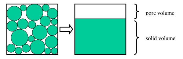
Figure 1: Definition of eigen-packing: eigen-packing = solid volume / total volume.
