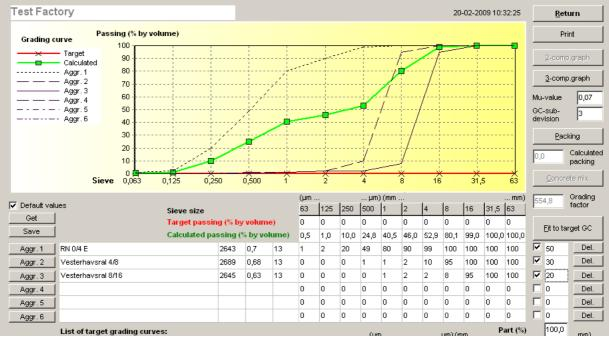
Figure 8. Combined grading curve and passing % (green curve and numbers) of the 50:30:20 % by volume combination of RN 0/4 E, Vesterhavsral 4/8 and Vesterhavsral 8/16.
