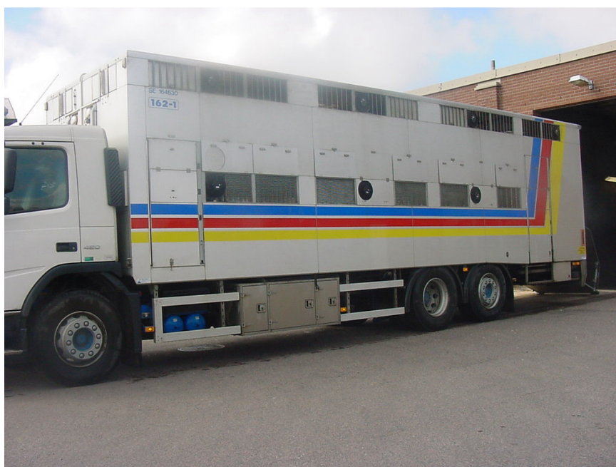
Figure 3 – Shows placing of openings for natural ventilation and the mechanical fans (1 per compartment).
