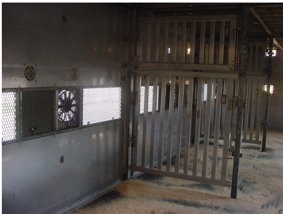
Figure 4 – Interior showing the ventilation openings and placing of the mechanical ventilation.
