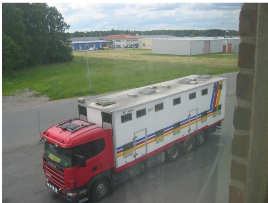
Figure 6 – Vehicle seen from the left and from above showing the openings in the roof.
