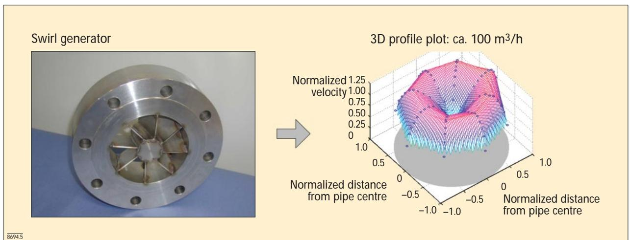
Figure 5. The applied swirl generator, and the resulting 3D LDV profile plot
