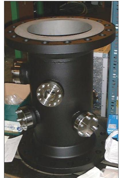
Figure 4. Window construction for use in on-site calibration of large flow meters
