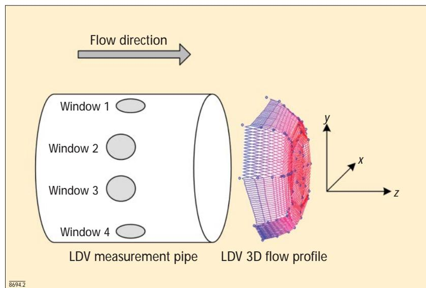
Figure 2. The generation of a 3D LDV flow profile from measuring point velocities across several pipe diameters
