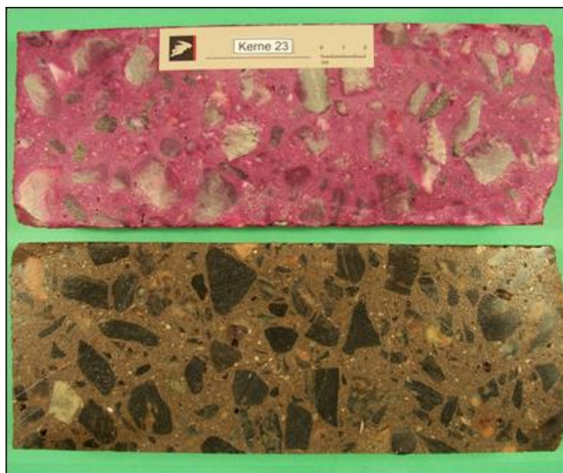
Figure 3. Surface of the concrete to the left. In the top image pH-indicator is sprayed onto the concrete to reveal carbonation. – no carbonation found.
