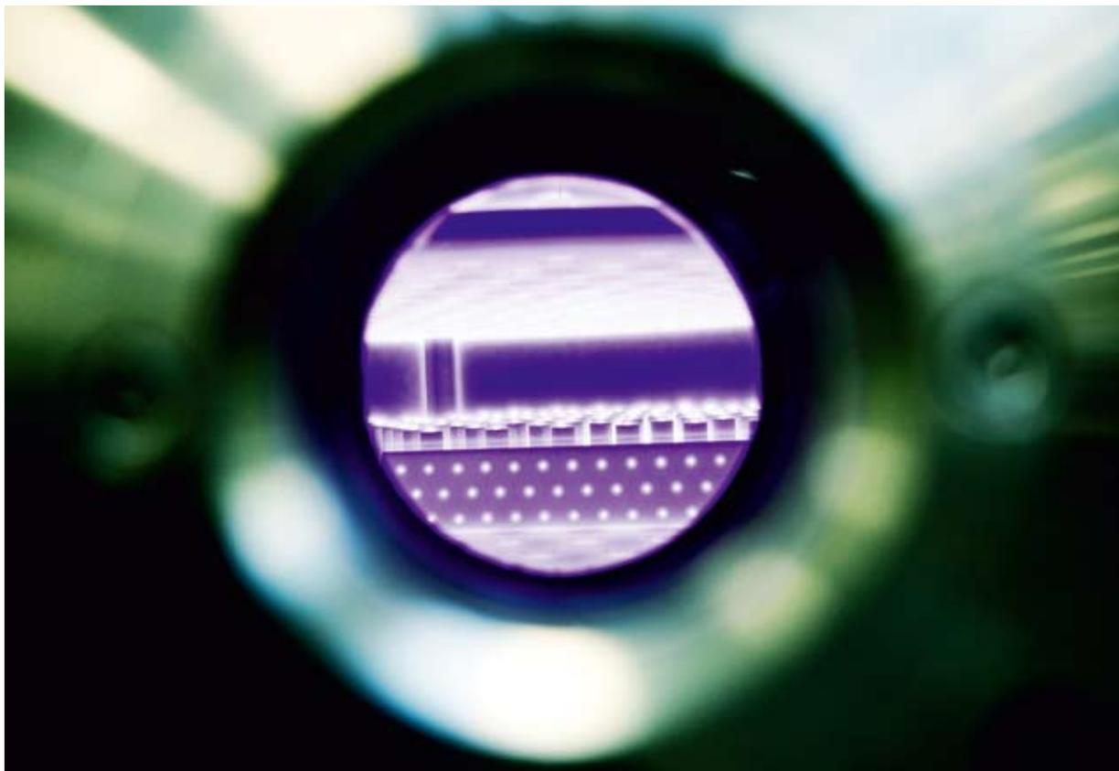
Plasmanitriding is a diffusion process in which nitrogen heated to temperatures of between 450 and 580°C diffuses into the metal surface forming a hard and durable layer.
