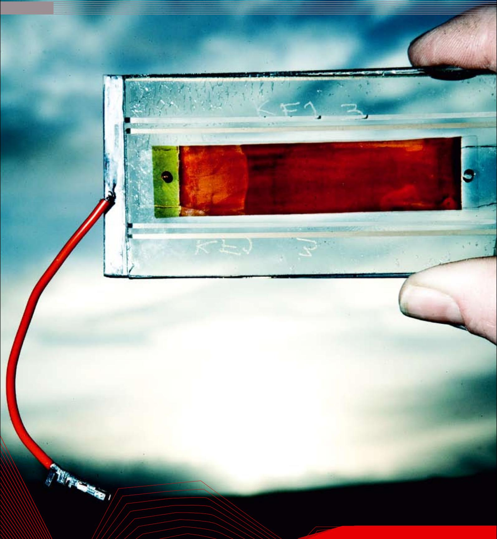
The Danish Technological Institute is a leading player in the research and development of electro-chemical solar cells in glass. The new type of solar cells is ideal for the decoration of buildings, also providing a pleasant interior climate.
