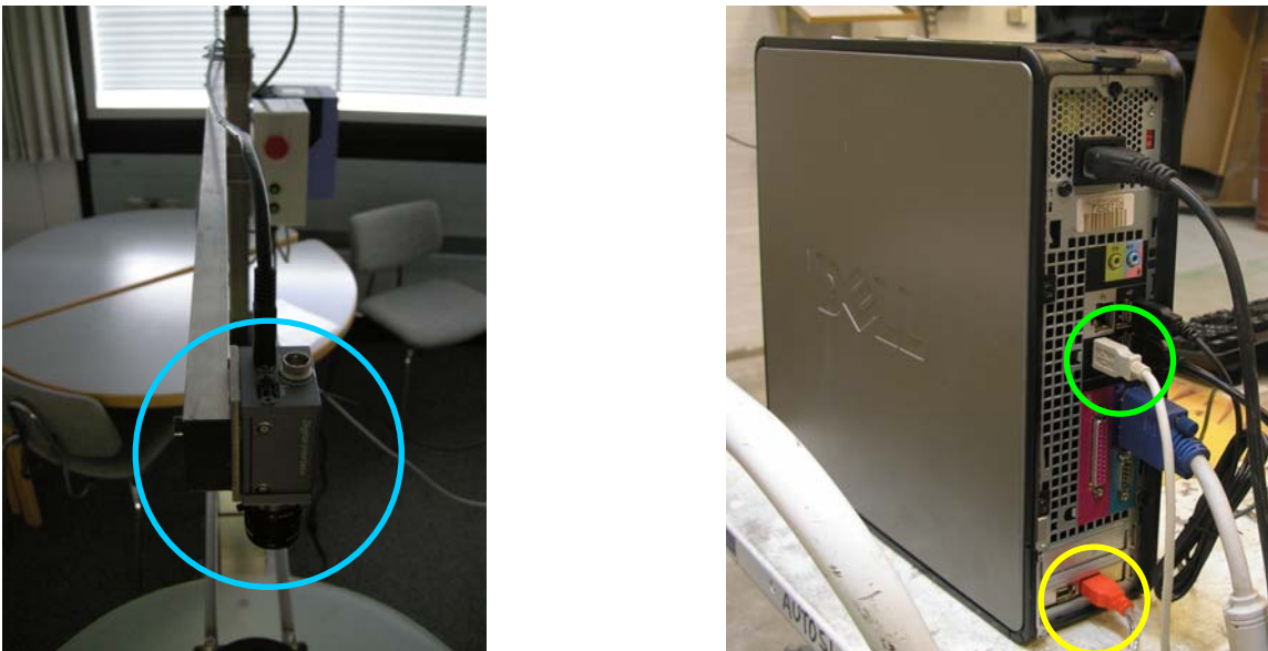
Figure 1. Left: Camera (in the blue circle) mounted on top-arm looking down towards the base plate. Right: Rear view of PC. Green circle = Lifting unit USB-cable. Yellow circle = Camera fire-wire cable.
