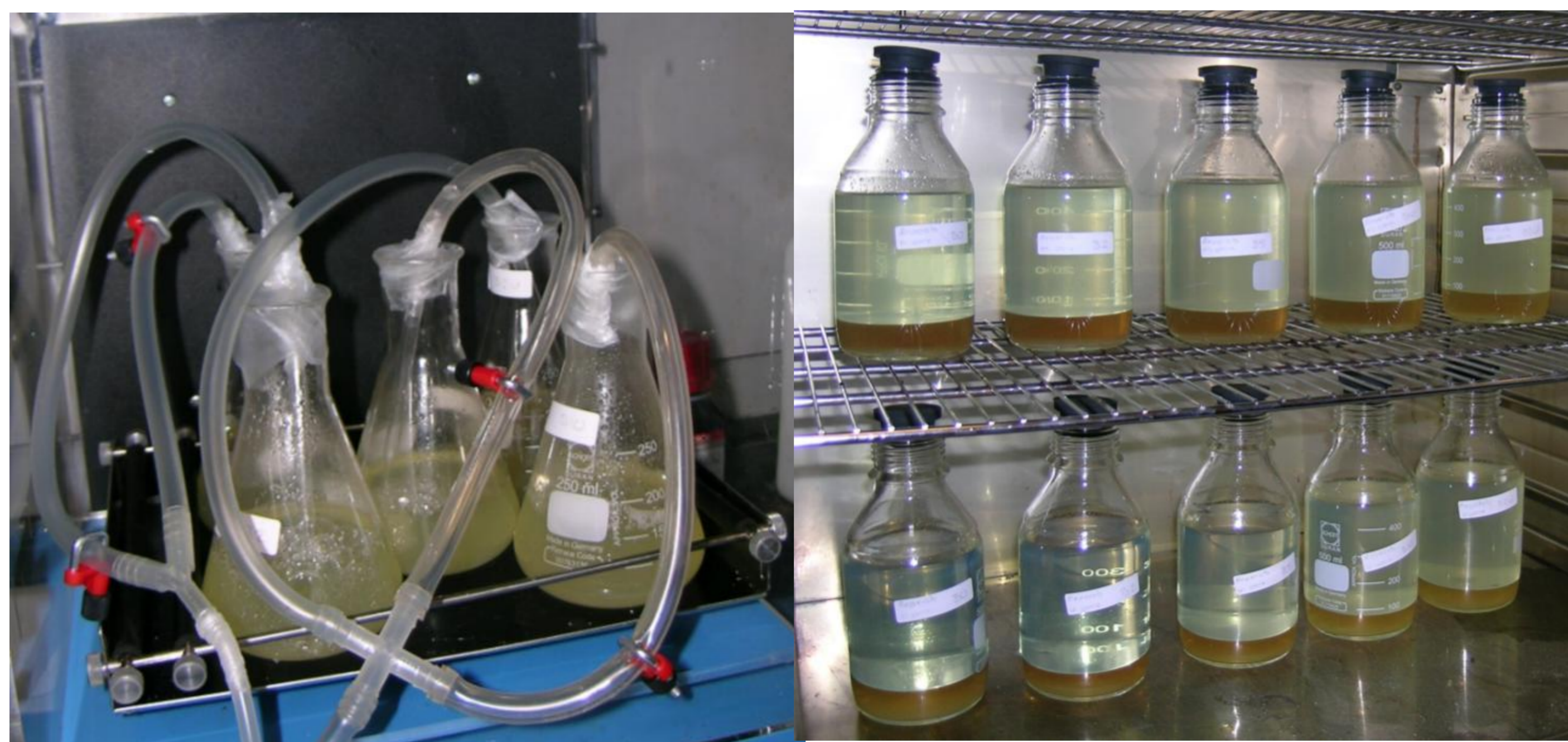
The photograph shows the aerobic experimental setup with the biodiesel blends (to the left) and the anaerobic setup (to the right).
