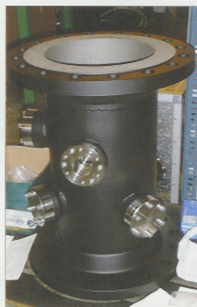
Figure 4. Window construction for use in on-site calibration of large flow meters
