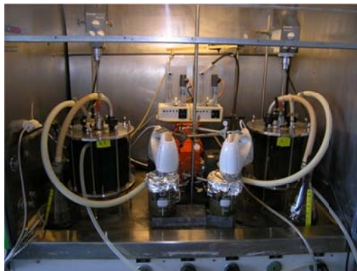
Fig. 3.8 Experimental setup for co-digestion trial
