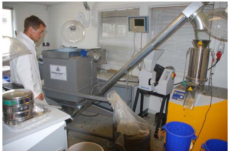
Fig. 4.11 Production of Ulva lactuca pellets on Amandus KAHL pellet press at Danish Technological Institute.
