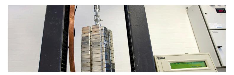
In our state-of-the-art force laboratory Danish Technological Institute performs accredited calibrations of most force measuring equipment on the market. We also perform accredited calibration of large testing machines at the customer's address.
