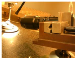
Camera to check fixture and set up for calibration
