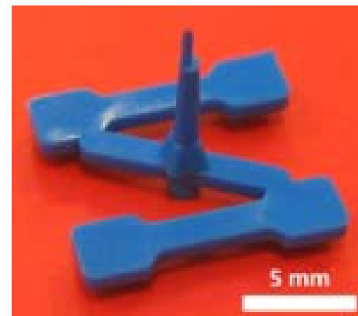
5 Dog Bones used for micro mechanical material tensile testing, made of acetal polyoxymethylene (POM). Part weight: 35 mg.
