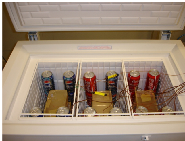
Figure 5: SolarChill-B chest-type prototype based on a 160 liter ice liner cabinet. The cooler is equipped with 5 baskets (3 upper baskets and 2 lower baskets). The photo shows that the cooler is tested with 12.5 kg test packages and 13.3 kg soft drinks (40 cans) simulating food and drinks.
