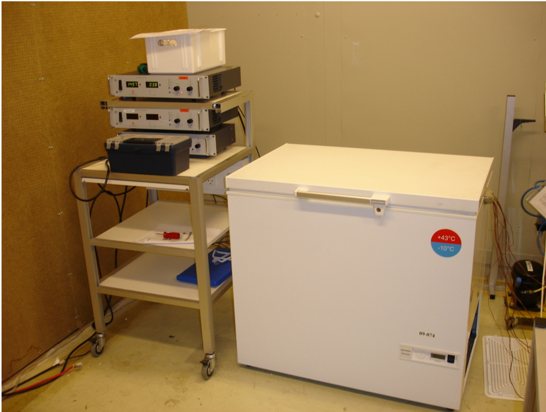
Photo: Test of SolarChill B in climate chamber at DTI. The cooler is powered by power supply (15 V) and power is available 10 hours a day. Temperatures are measured and recorded (8 temperatures inside the cooler and ambient temperature and humidity)
