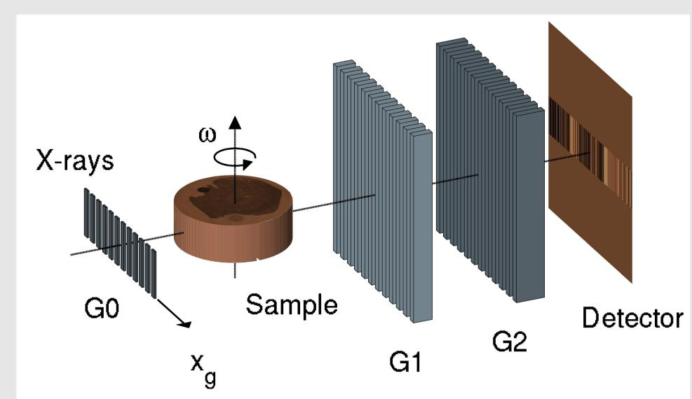
At laboratory-based setups a third grating, G0, is included to assure satisfactory coherence in the x-direction. A rotation sample stage can be included for tomography.
