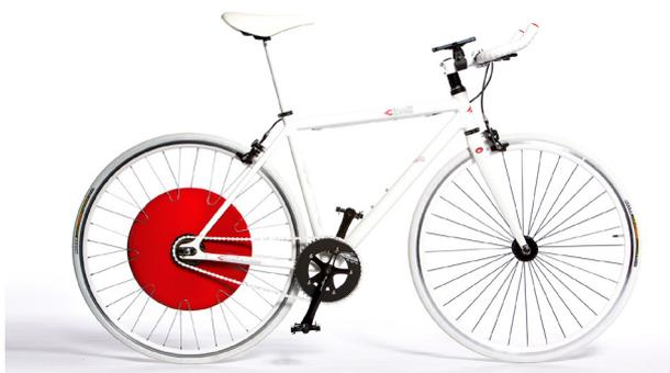
The Copenhagen Wheel – first announced by MIT's SENSEable City Lab in 2009 – became available to the public in November 2013. Cyclists replace their rear wheel with the Copenhagen Wheel, which then automatically assists with pedaling via an on-board motor. Battery power is generated from braking and cycling downhill. Users can adjust the assistance rate via the Superpedestrian cellphone app, which also collects information on congestion, air and noise pollution and road conditions.
