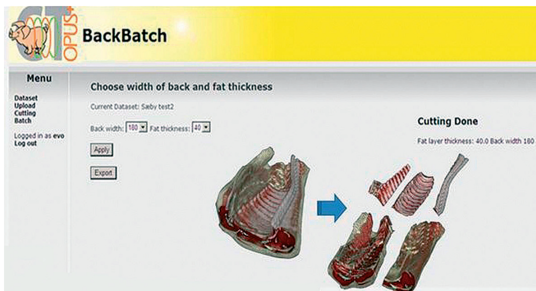
Fig. 6: Virtual cutting of products from the middle piece. The width of the back and the thickness of the fat layer are determined by the user and transferred automatically to all model pigs. A data file containing detailed information on weights and yields is created.
