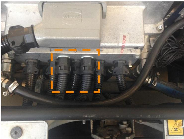
Figure 3.3.3: Upper cable conduits are retrofitted for DC connector
