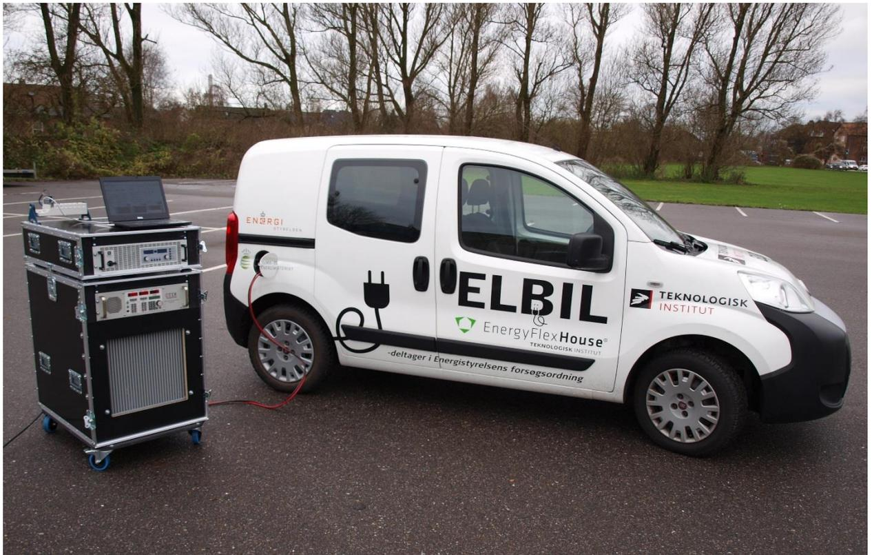
Figure 3.2.1: The mobile load bank in action on parking lot in Aarhus, Denmark
