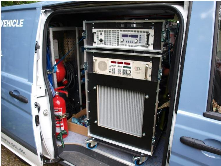
Figure 3.3.1: Mobile load bank unit in the battery service vehicle
