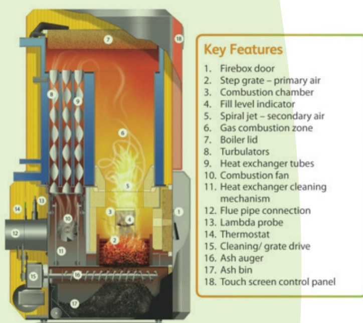
Figure 3. Set-up of a modern biomass boiler, with fan and lambda sensors. As an example a Guntamatic Powerchip boiler [3]
