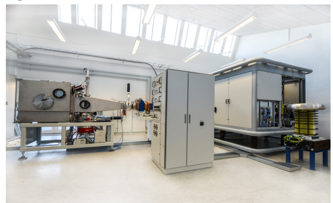
Figure 2: Danfysik 1090 high current ion implanter.
