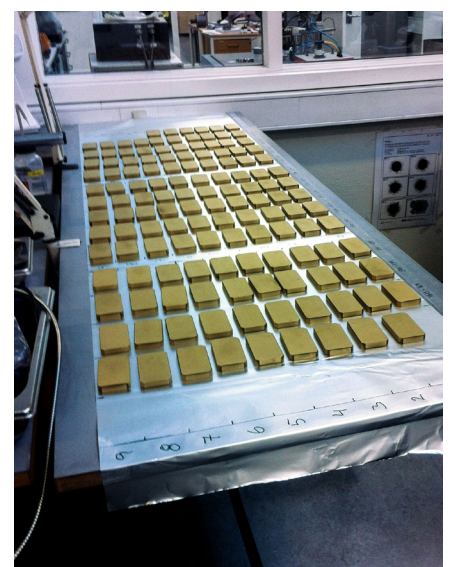
Quality control of neodymium magnets PVD coated with TiN.
