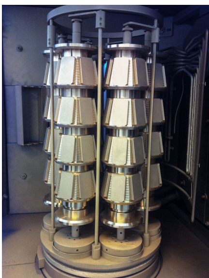
TiN coated neodymium magnets ready to be debatched.
