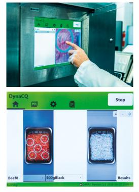
DynaCQ marks contaminant objects with a halo, here shown in a tray spiked with fragments of soft and hard plastic and earplug.
