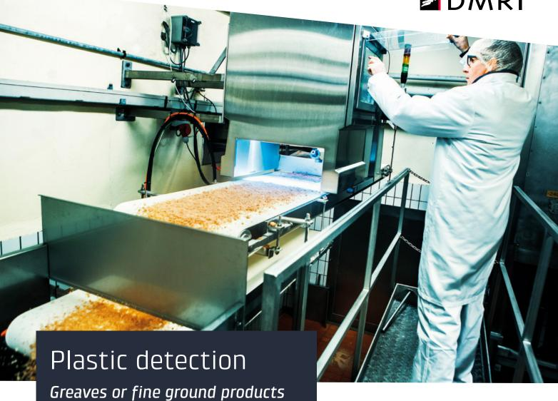
**DynaCQ** provides on-line inspection of your greaves or fine ground products to ensure they are free from contamination
