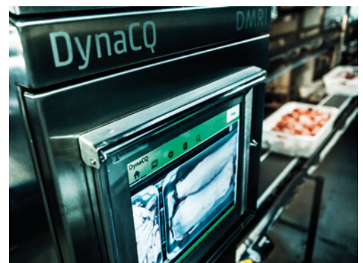
DynaCQ measures product content in crates to check for contaminants and to determine content and automatic destination
