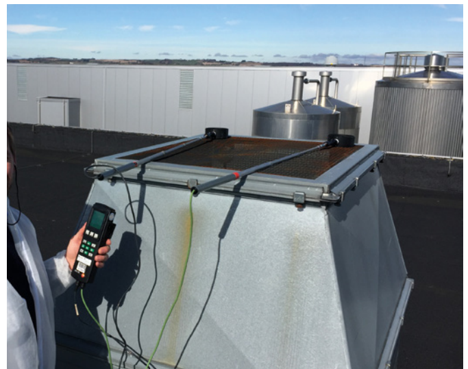
On-site air flow measurements
