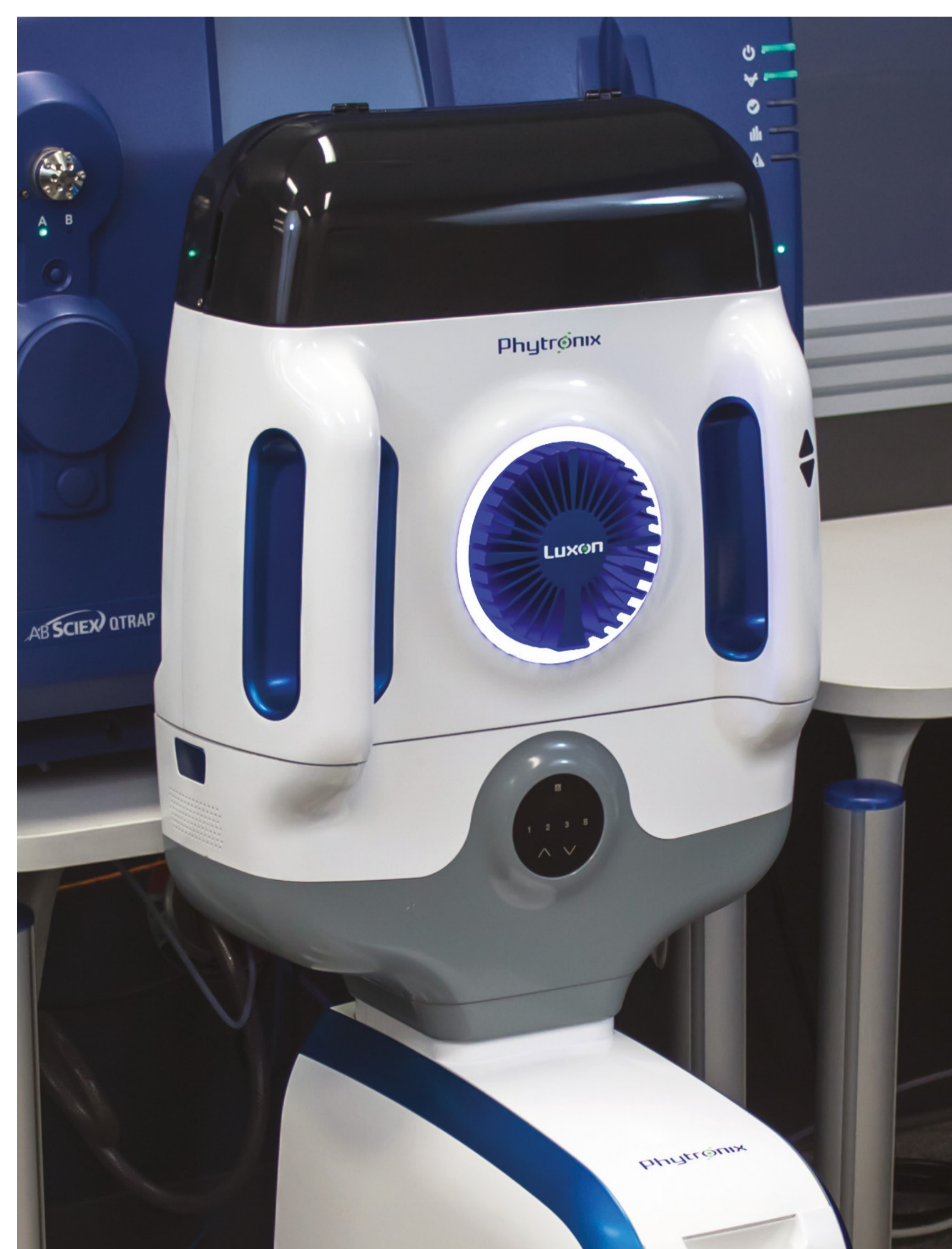
Figure 2. LDTD in the Luxon version front-ending a Sciex MS-MS. The Luxon LDTD can be automatically loaded with Lazwell plates by a Scara robot.
