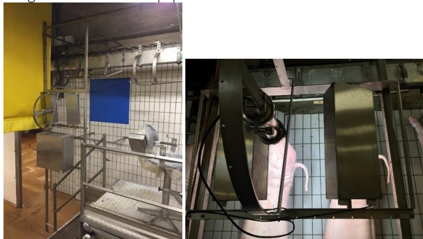
Figure 1. Photo of the TailCam equipment at the slaughter line.
