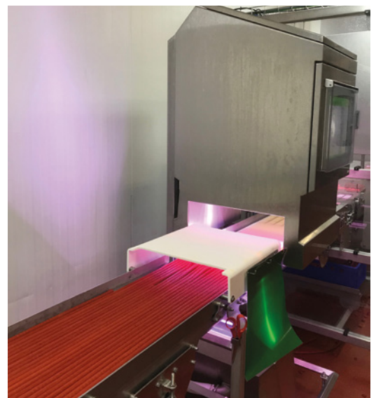
Two side screening of sausages for plastic casing remnants.
