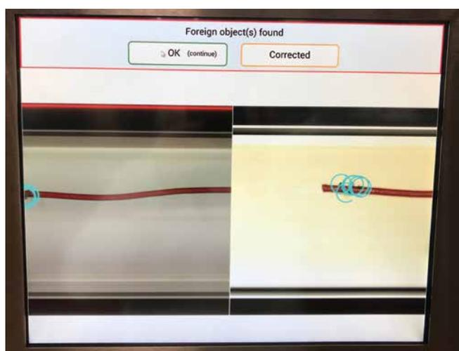
*DynaCQ marks the detected casing remnants with a halo, and stops the belt and product, at a fixed position for manual removal.*
