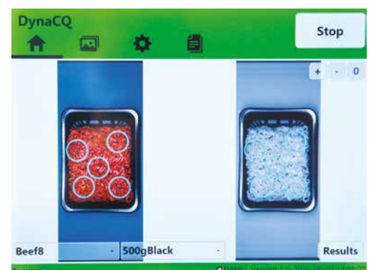
DynaCQ marks contaminant objects with a halo, here shown in a tray spiked with fragments of soft and hard plastic and earplug.
