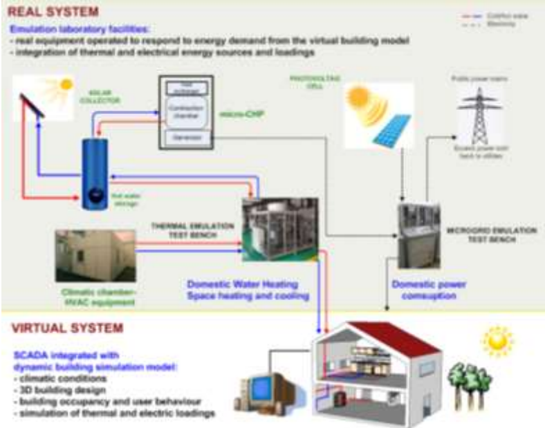
Figure 6. The general layout of the Semi-virtual Energy Integration Laboratory test facility at IREC, Spain [5].
