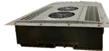
Baseline R407C unit for high-speed rail passenger car AC
